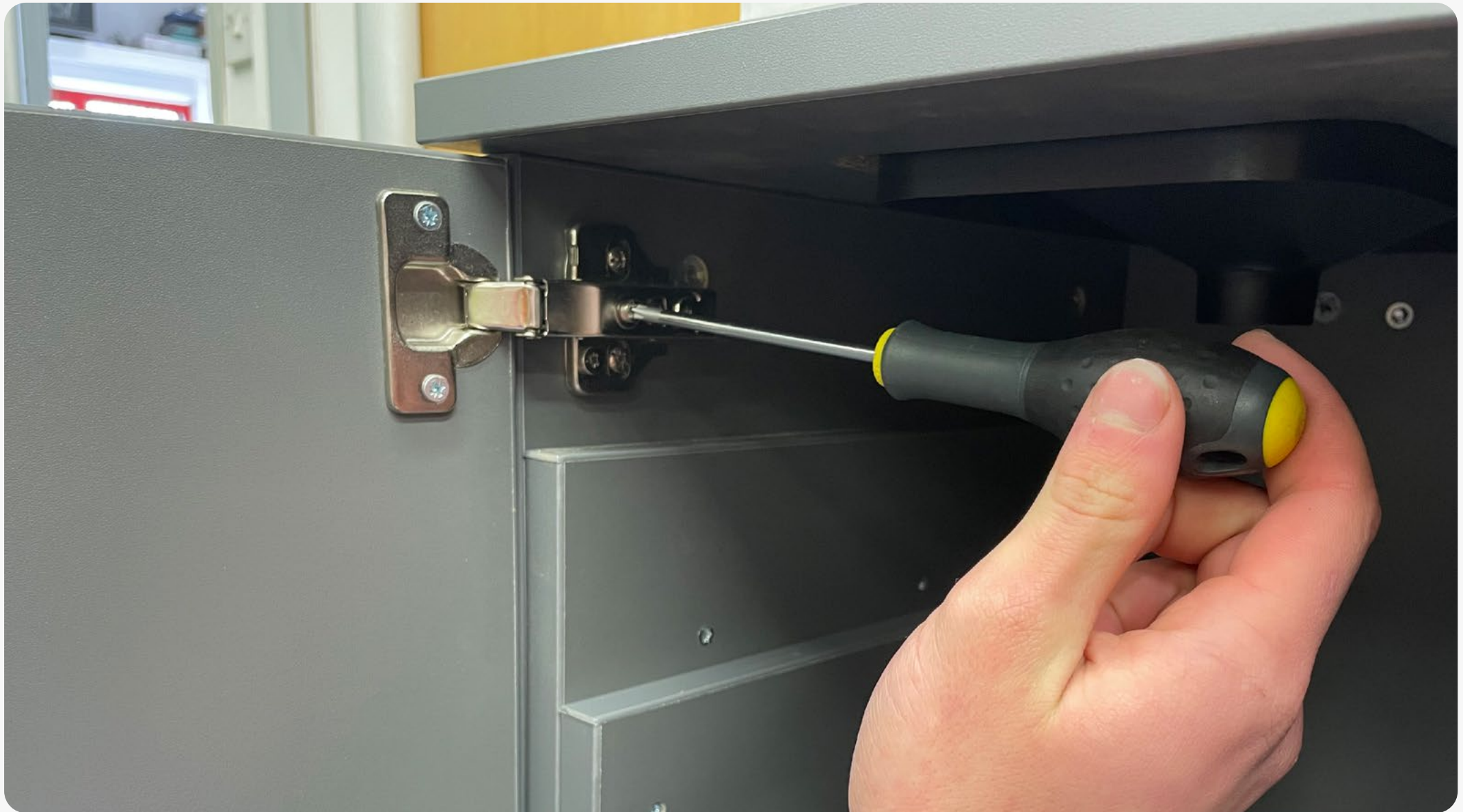
2 Open the door and turn the front screw on the hinges clockwise to shift the door towards the center of the unit.
