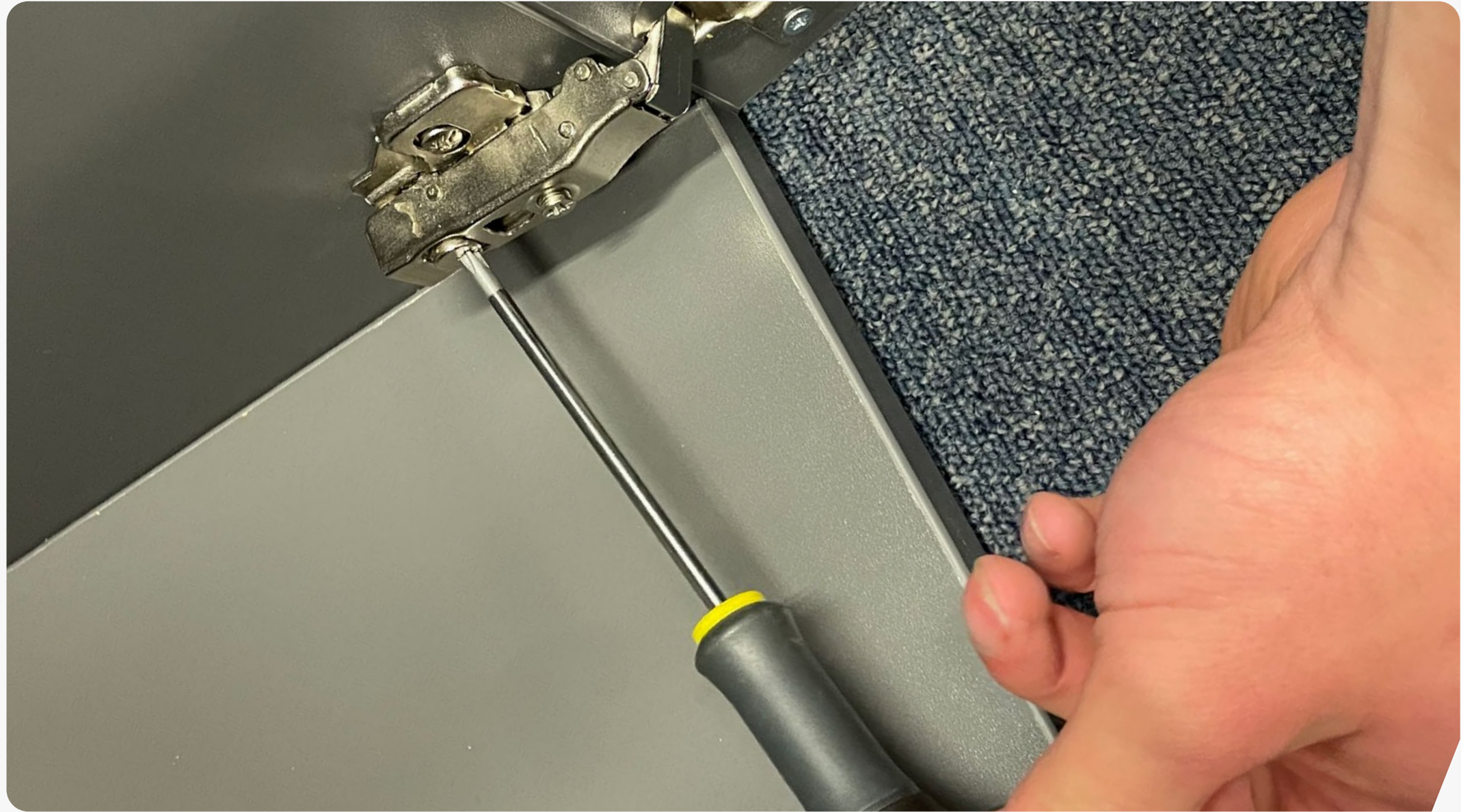
3 Turn the rear screw counterclockwise if the door requires adjustment to move away from the center of the unit.
